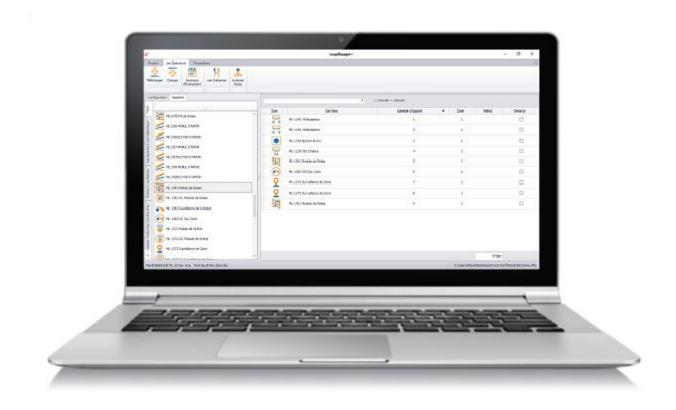
**ML-1612** LoopManager+ is a computer program for programming ML-12XX series fire alarm control panels. With the LoopManager+ program, devices settings (location name, zone, delay, etc.) and panel settings (panel name, operating mode, etc.) in the fire alarm system can be made. Panels can be programmed as one by one or all panels in network structure can be programmed via any panel.
