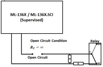
In case of open circuit, the resistance seen at the switch monitoring input will be read as " $R_T = \infty$ " and the module will transmit the open circuit fault signal to the panel.
