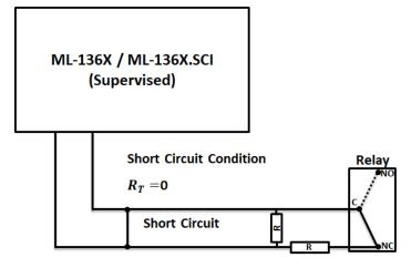
In case of short circuit, the resistance seen at the switch monitoring input will be " $R_T = 0\Omega$ " and the module will transmit the short circuit fault signal to the panel.
