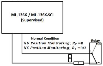
In its normal state, the resistance seen at the switch monitoring input will be read as " $R_T = R$ " when the monitored relay is in "NO" position, as " $R_T = R/2$ " when it is in "NC" position, and it will be detected by the system that there is no break, short circuit, etc. in the monitoring line.
