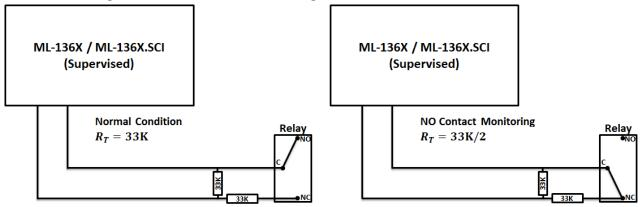
\* When the resistance seen at the switch monitoring input is " $R_T = 33K$ " in the normal position, the resistance seen when the monitored relay changes position will be " $R_T = 33K/2$ " and the information that the relay has changed position will be transmitted to the panel.
